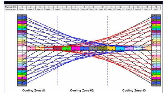
The Isolated Dual Star Switch Architectures are generally implemented as custom ATCA backplane designs. In such systems, the up-time performance and the 5-9's reliability are the overriding requirements. The absence of a single point of thermal failure is the major difference between the standard switch and custom ATCA architectures.
